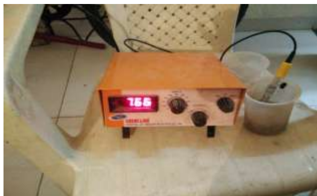
Fig. 6. pH Test of concrete
